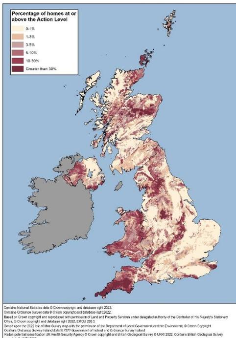
**Figure 2:** The amount of radon in the ground depends on the geology, which helps us to produce a radon potential map by combining geology data with the results from radon measurements in homes. The areas at highest risk are called radon Affected Areas – more detailed maps and information are on [www.ukradon.org](http://www.ukradon.org).
