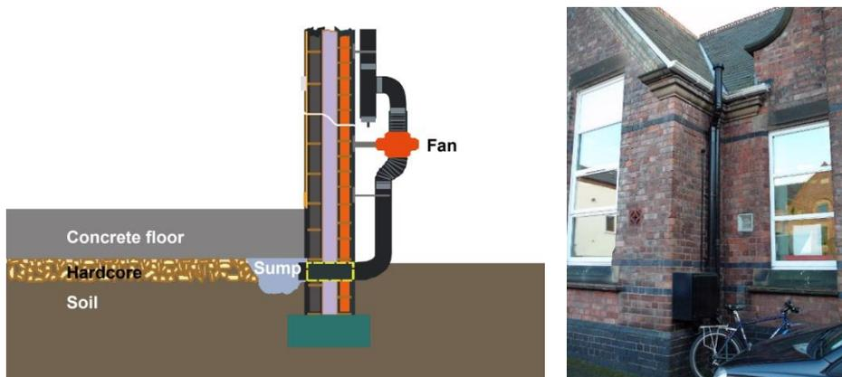
**Figure 3:** A radon sump and pump is a low-pressure zone under the floor that diverts the radon-laden air away from the room with a pipe and fan, and vents it to the outside. The pipework design can integrate well with the building. Such a system is usually effective for an area of up to 250 m<sup>2</sup>. Other mitigation methods include ventilation under suspended floors.
