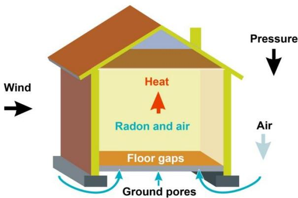
**Figure 1:** Radon is drawn into buildings through gaps in the floor and cavity walls, by warm air rising. Radon levels will vary between neighbouring buildings and from room to room, according to the size, design and usage
